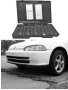
Figure A-23. Road Side Spike Strip
